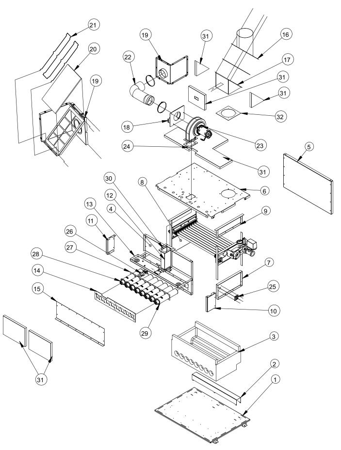
Figure 20. Combustion Chamber Components.
